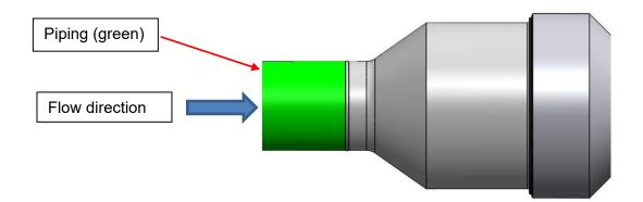
Prevent any bending and shearing stresses during and after welding. Weld very carefully to prevent any deformation of the valve. Weld heat input should be as little as possible.
